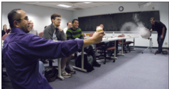
Jon Jacobsen and Francis Su demonstrate the fluid dynamics of a vortex cannon (the stable toroidal ring will blow out the candle Su is holding). Many HMC math faculty use physical demonstrations in their lectures.
