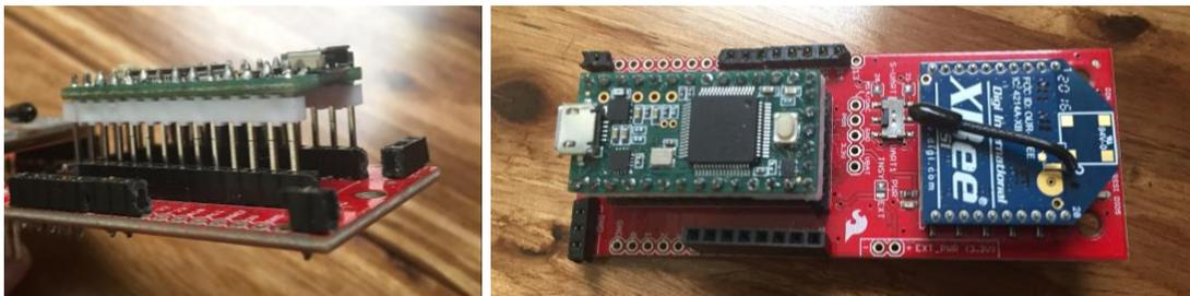
Figure 7: Side view of the Teensy with male header pins soldered to it, connected to female header pins soldered to the Teensy/xbee breakout board (a). In (b), a top view of adapter board with female header pins, Xbee, and Teensy attached
