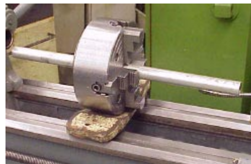
Figure 4. Use the bar technique to lift heavy chucks.
