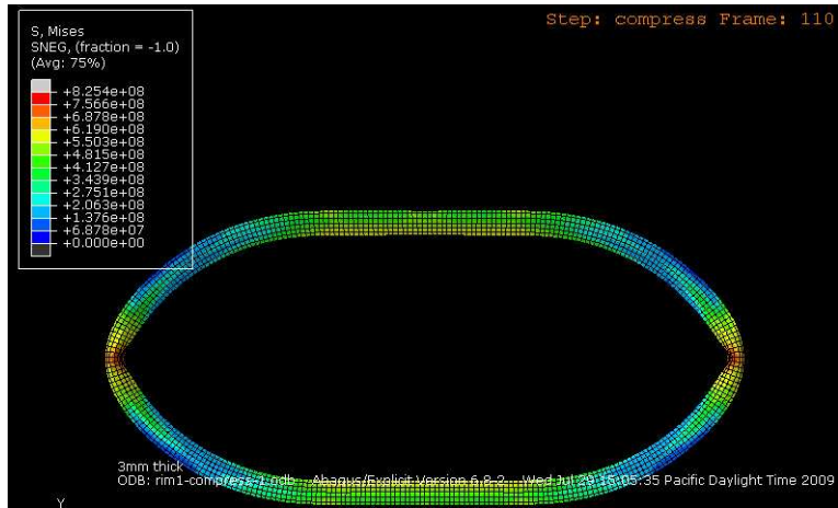
Figure 10: Rim1 Under Compression
