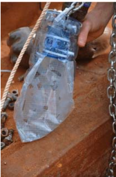
Fig. 19. Funnel structure to guide the harpoon inside the pipe.
