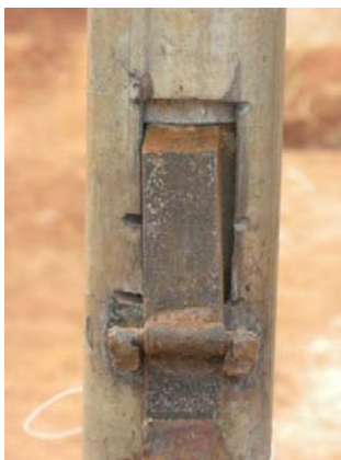
Fig. 5. The rocket's pawl caught beneath the pipe coupling
