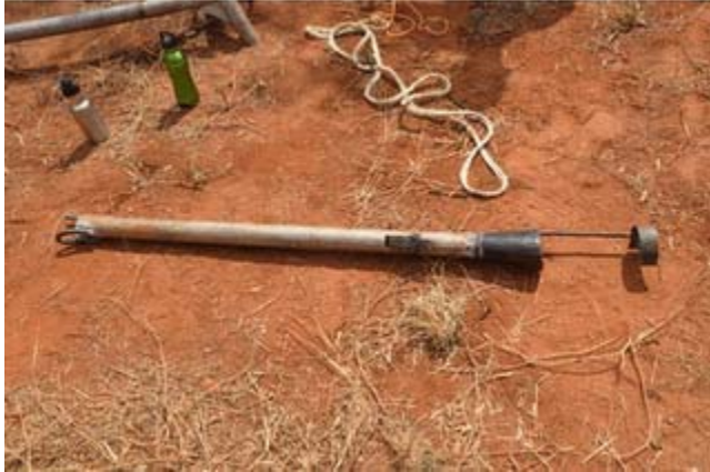
Fig. 4. Final pipe-retrieval design. The “rocket” is made to fit around the pipe. The curved structure at the right is designed to pull the top of the pipe away from the wall, and the dark portion is a funnel to guide the pipe into the rocket. The pawl on the side is designed to lock below the first pipe coupling.
