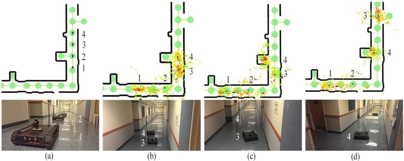
Fig. 6: Jaguars performing a swap in hardware and the graphical interface, where nodes are represented by dark circles and walls are depicted by solid lines. Robots were positioned in the hallway on distinct nodes. In (a), robots start lined up. Next, Robots 1 and 2 move down the hallway (b), while 3 and 4 begin a swap. In (c) Robot 4 moves out of the way of Robot 3. In (d) Robot 3 moves past and the swap is complete. All robots have reached their goal.
