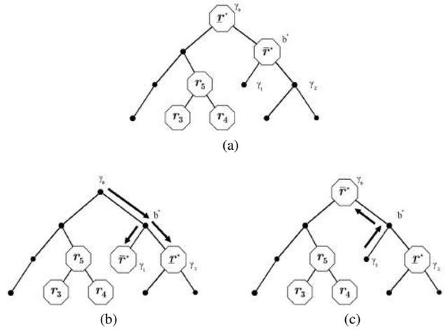
Fig. 4: *Process of finishing a swap*. In (a), the robots  $\bar{r}^*$  and  $\tilde{r}^*$  have just arrived at an available branch node  $b^*$ . In (b),  $\bar{r}^*$  and  $\tilde{r}^*$  arrive at their respective twigs  $\gamma_1$  and  $\gamma_2$  (c) shows  $\bar{r}^*$  and  $\tilde{r}^*$  after the swap with positions reversed.
