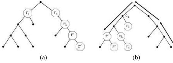
Fig. 3: *Swap suppression at child of  $g(r_s)$* . In (a), two robots  $\bar{r}^*$  and  $\tilde{r}^*$  initiate a swap that takes them to the other side of the tree, where they push two unsolved robots,  $r_4$  and  $r_5$ , and one solved robot  $r_s$ . In (b),  $r_s$  is waiting for the return of the swappers before moving back to its goal  $g_s$ , preventing it from becoming unsolved.
