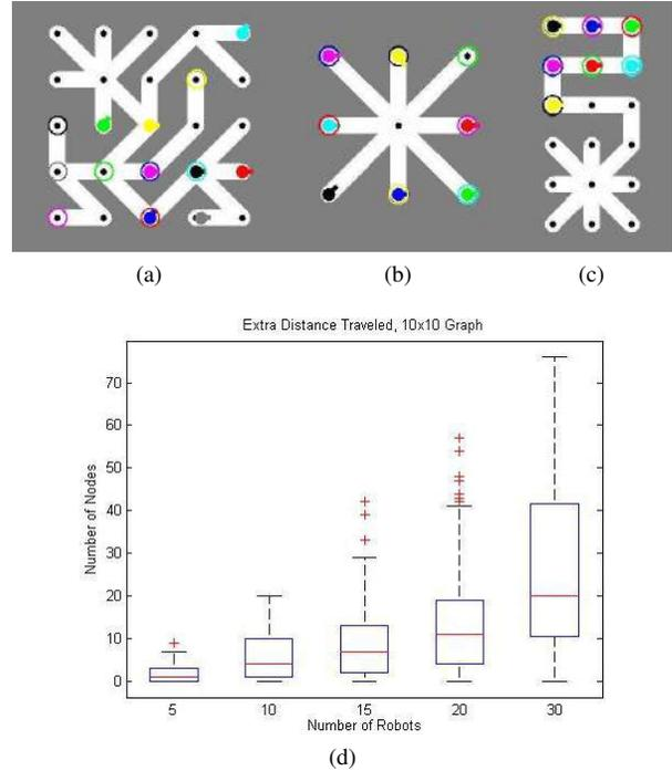
Fig. 5: PSW Performance: In (a), test cases with 10 robots in a randomly generated 5x5 grid, with more difficult cases in (b,c). In (d), extra distance is (Number of nodes traversed) - (Number of nodes on the direct path from start node to goal node). The red line indicates the median number of nodes and the blue box illustrates the interquartile range.
