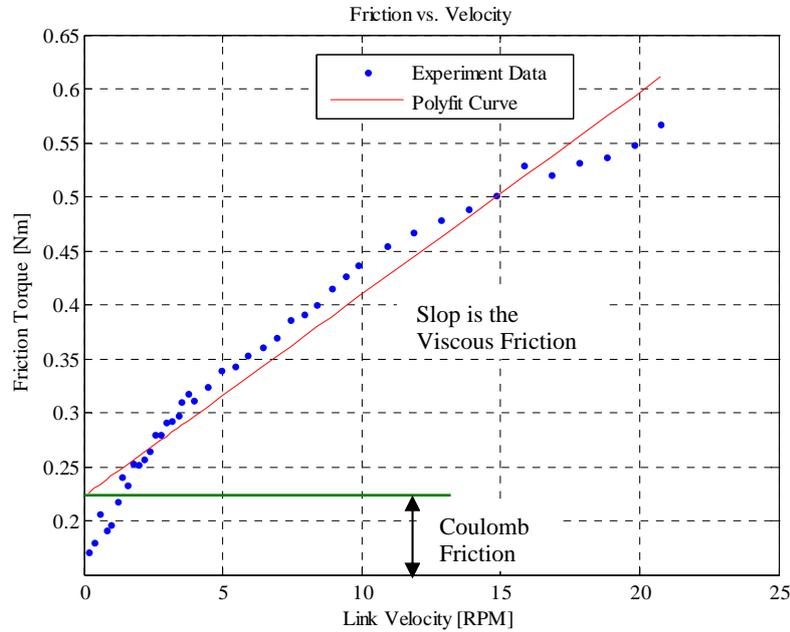
Fig. 6. Harmonic drive friction experimental data and curve fitting
