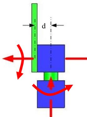
**Fig. 1.** 2DOF Robot with cubic joint (“d” is the link offset)
