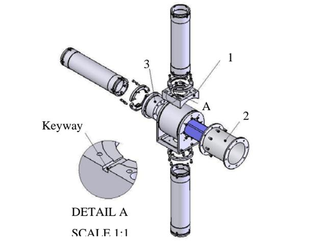
**Fig. 2.** Proposed joint module with links
