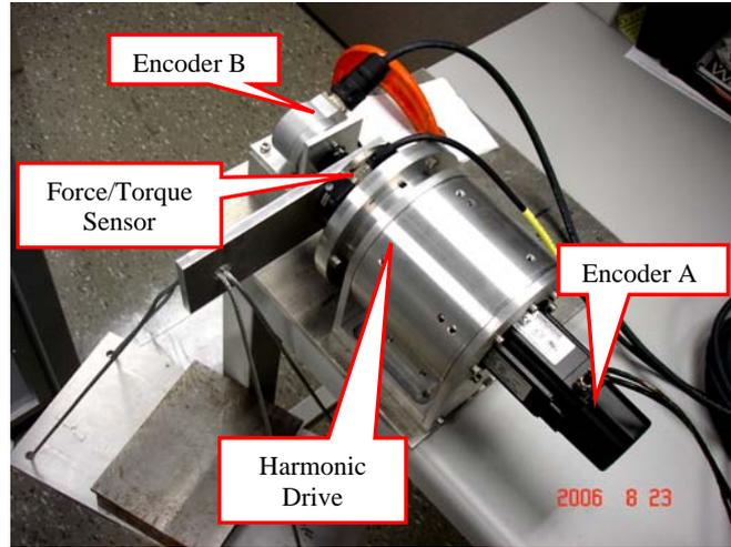
**Fig. 4.** Experimental setup for HD flexspline compliance calibration
