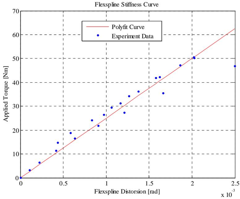
Fig. 5. Flexspline stiffness experiment data and curve fitting
