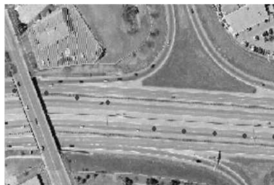
Fig. 7. An example of GPS Error while traveling on a highway (Dark dots represent GPS readings)
