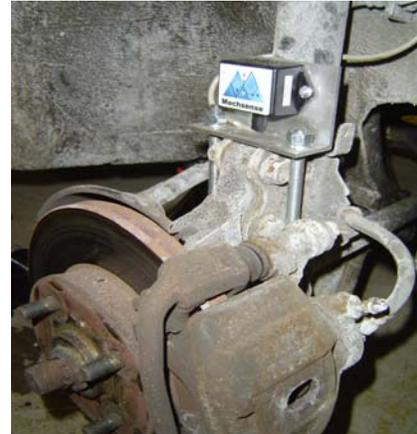
**Figure 3 Accelerometer mounted on the bottom of a damper to measure the vertical acceleration of the wheel hub**
