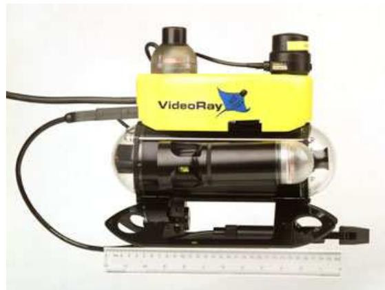
Figure 11: The VideoRay Pro III Micro ROV.
