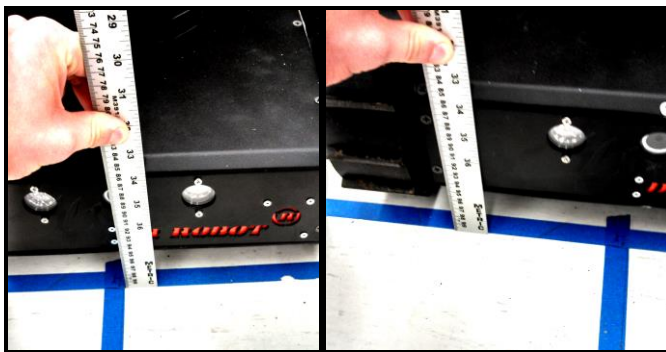
Fig. 10. Alignment of the Jaguar Robot to the coordinate frame. Center alignment (left) and side alignment (right).
