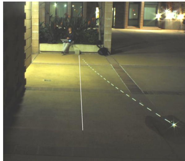
Fig. 2. Trajectory of the Jaguar over 20 seconds exposure photo. Each dash represents 0.25 seconds. The white line down the center is the robot’s estimated path.
