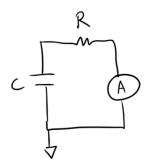
This obviously is not a practical way of measuring voltages but it does illustrate the key properties of a good voltage meter: it goes in parallel with the voltage being measured and it draws no current. Yes our capacitor did draw some current at the start but when it got up to the full voltage it did not.
