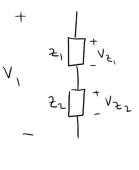
$$V_{Z1} = \frac{V_1 Z_1}{Z_1 + Z_2}$$
