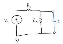
A capacitor is like a water tank and so when I first insert it next to the element in the circuit it will suck up all of the current but as the charge on the capacitor increases the current is requires will drop to 0.
