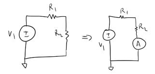
Well we must place the meter into the path of the current. If the current does not flow through our meter then it will not create the magnetic field we need.
