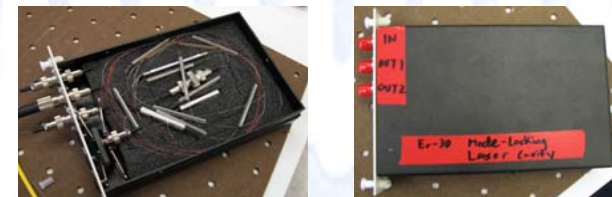
Figure 6: Final laser cavity in packaged form, SAM stabilized with glue and foam padding.
